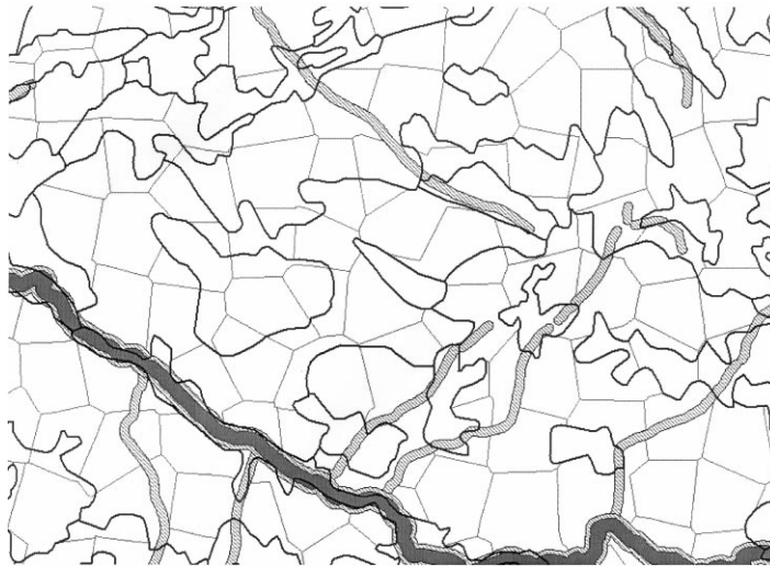
Fig. 3. An example of the simulation polygons created through the overlay of forest cover polygons (heavy lines) and other planning zone boundaries (riparian reserves — dark shading, and riparian buffers — hatched), followed by a Voronoi tessellation (light lines). Simulation polygons are created from the intersection of all boundaries. Note that slivers less than 1 ha (user-defined) created by the Voronoi tessellation have been recombined with the adjacent polygon with similar characteristics. The tessellation also does not affect those polygons that initially are less than 2 ha (user-defined). This figure is only a small excerpt from a much larger landscape.
